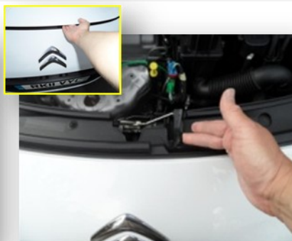
Push exterior safety catch and raise bonnet
