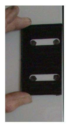
The outer holes (Arrow A) should be 1.85 inches (47mm) away from the edge of the door.
