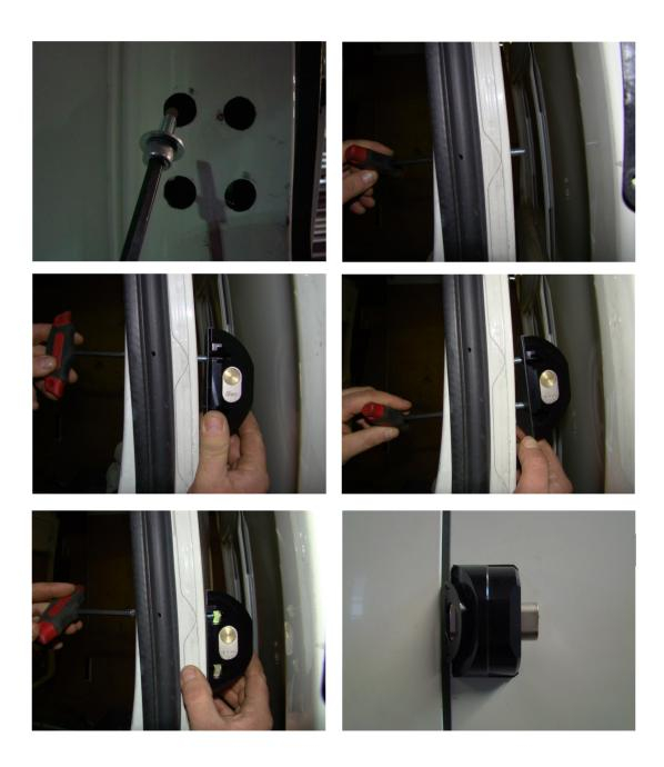
Place the left gasket in line with the fitted lock and draw two circles at either end of the gasket, these are the drill holes. The edge of the gasket should be in line with the door edge.
