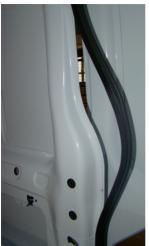
On the body panel, place the gasket 9.84 inches (250mm) up from the door runner (shown by the arrow) and draw two circles at either end of the gasket, these are the drill holes.
